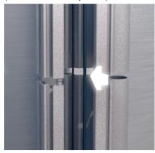
When the trolley on which the device is mounted reaches the operating dimension, it automatically hooks in position by means of a metal **locking system**; from this moment on, the equipment is ready for operation.
