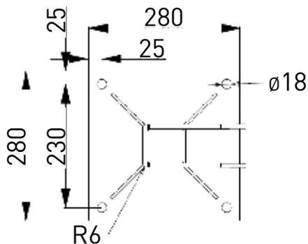
The represented concrete foundation is indicative. It must be calculated based on the type of soil. The foundation is not required if the fixing is over a steel support.
