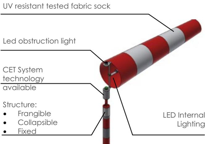
The internal lights of the sock and the obstruction light are powered by the innovative CET (Contactless Energy Transmission) system, for the wireless transfer of energy from the fixed to the mobile rotating part of the sock.
