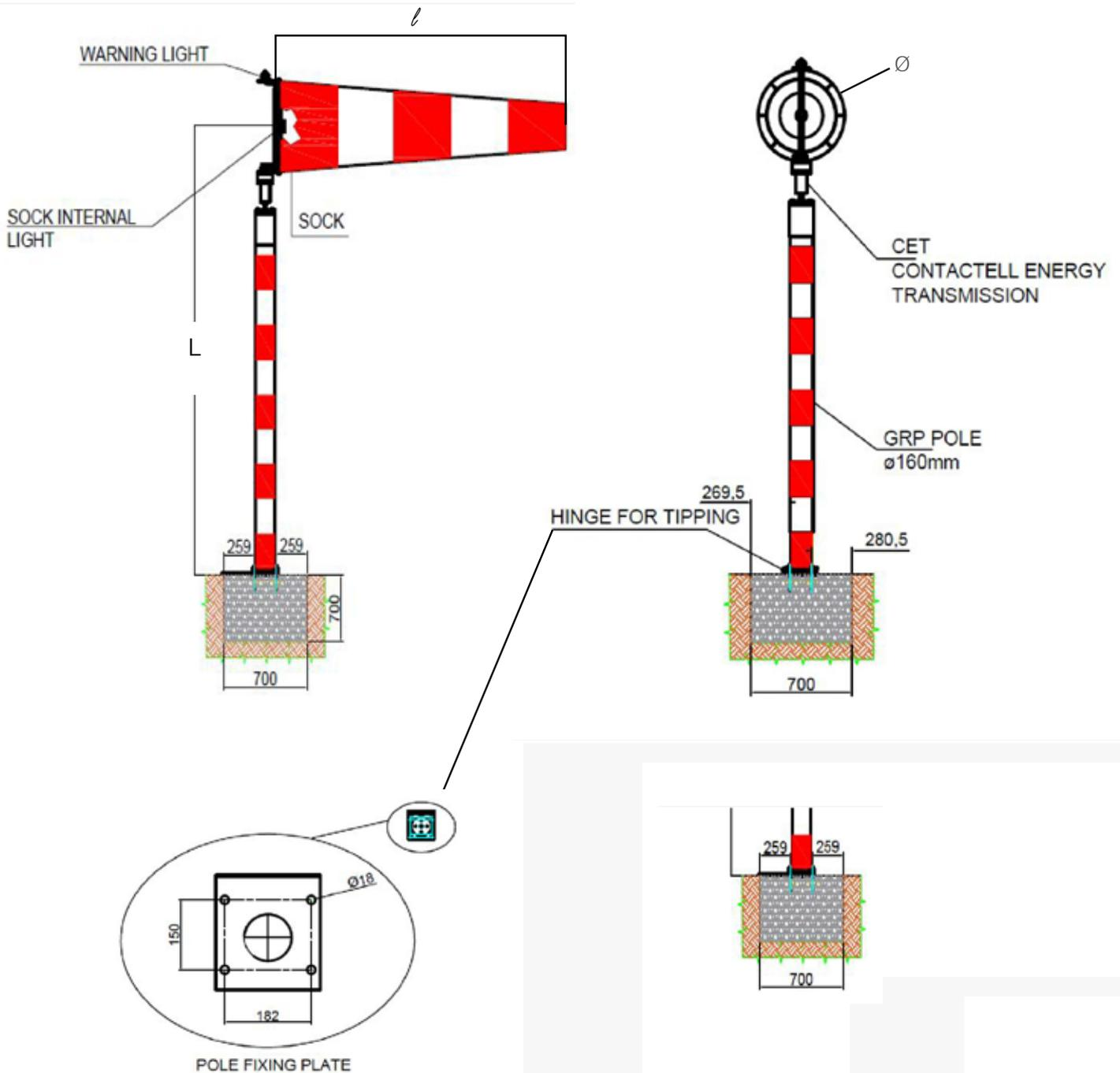
The represented concrete foundation is indicative. It must be calculated based on the type of soil. The foundation is not required if the fixing is over a steel support.
