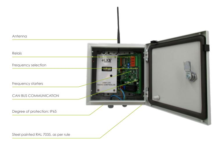
**L854-LXS** device lets the pilots turn on and control the heliport lighting system.
