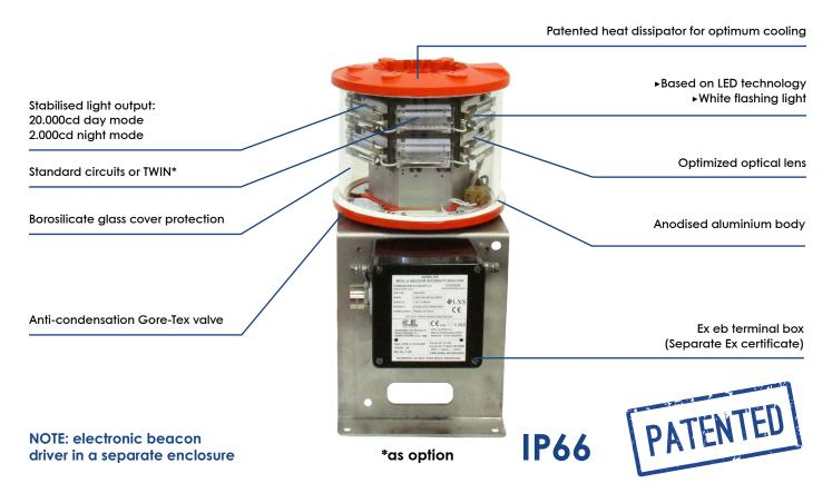
LUXSOLAR® L865-LXS Medium Intensity Obstruction Light is compliant to ICAO (Medium Intensity - Type A), FAA (Type L-865), ENAC and EASA compliant.
