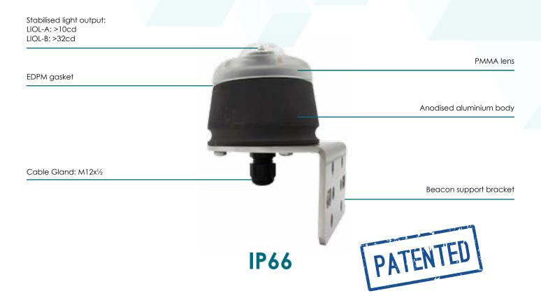
LUXSOLAR L810-LXS-ONE Low Intensity Obstruction Light is compliant to **ICAO** (Low Intensity - Type A or B), **FAA** (Type L-810) and **EASA certified.**
