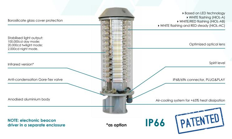
LUXSOLAR L857-LXS-200 High Intensity Obstruction Light is compliant to **ICAO** (High Intensity - Type B) and **FAA** (Type L-857). With a **body designed for optimum light emission and increased cooling, high quality and ultra-bright LEDs and patented lenses; LUXSOLAR HIOL-B product is the <b>most up-to-dated and technologically advanced Aircraft Warning Light.**
